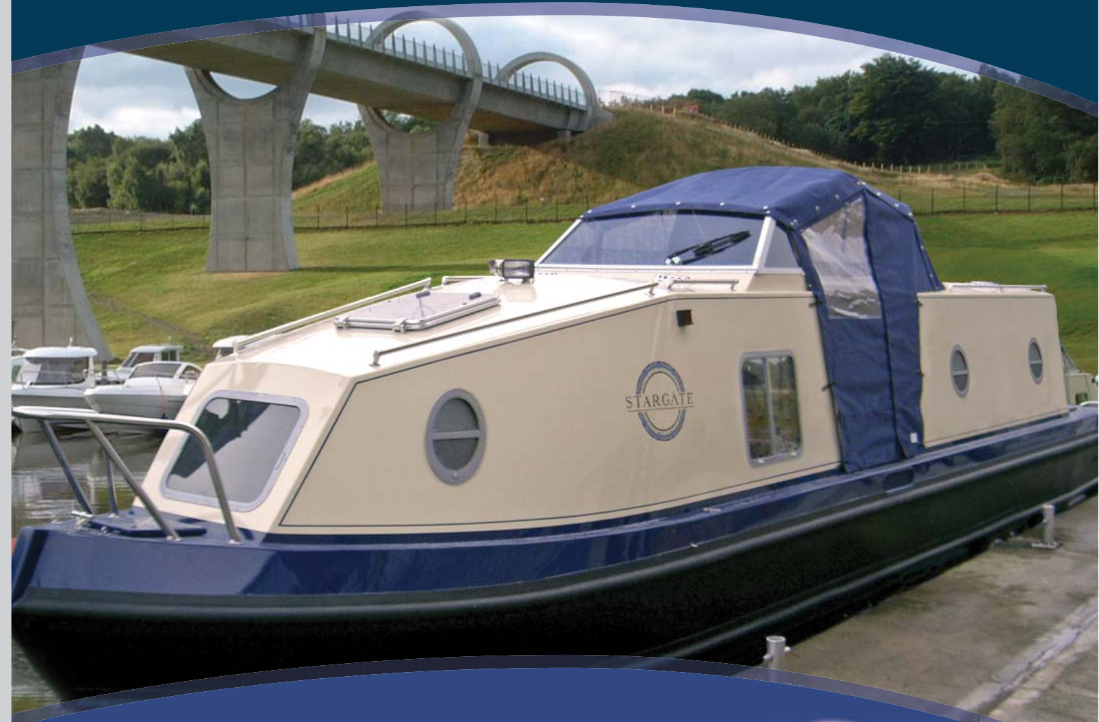
▲ The Sea Otter river cruiser is a 6.7m (22ft.) vessel with a 2.1m (6ft.10in.) narrow-beam.
